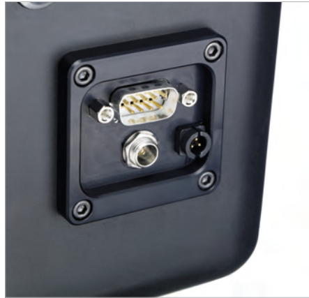
Computer Interfaces of the LasPaC II-P
